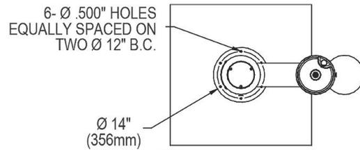
**SANITARY FREEZE-RESISTANT VALVE GROUND INSTALL DETAIL**
